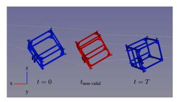
Fig. 1: Vizualisation of a path of the CDPR CoGiRo, parametrized by [0,T]. The first and last poses of the path are valid (blue). The continuous tension validation has found a non-valid pose (red) at parameter  $t_{\rm non-valid}$ , therefore the path is not valid. Cables (grey) are shown only for the red pose.
