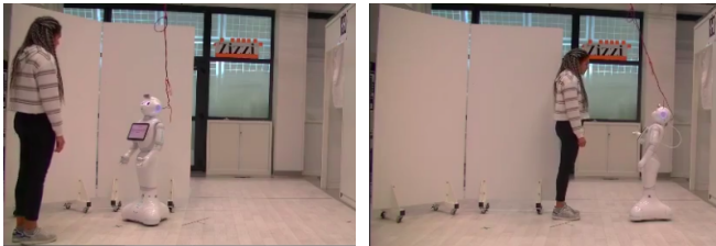
(a) Initial positions of the human and the robot. The human asked the robot where is the shop “Zizzi” (not visible to them because of the panels). (b) The robot and the human are in their final positions as planned by the robot. The robot is pointing to the shop direction which is now visible to them.
