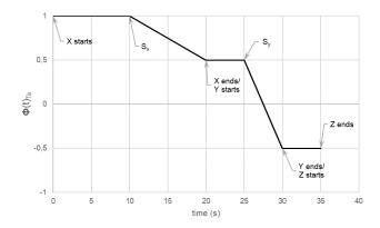
Fig. 1. Plot of  $\Phi(t)_{Ta}$  for a task composed of a sequence of three subtasks X,Y,Z with  $SD_X=10s,V_X=0.5,SD_Y=5s,V_Y=1,SD_Z=10s$  and  $V_Z=1$ . The duration of X exceeded  $SD_X=10s$  and reached 20s, the duration of Y exceeded  $SD_Y=5s$  and reached 10s, finally the duration of Z was less than  $SD_Z=10s$
