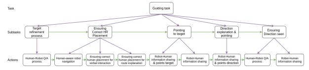
Fig. 3. The representation of the guiding task as a hierarchical task network with task, substasks and actions levels, exhibiting its incremental refinement into a sequence of HR interactive actions. Decomposition links are drawn in purple and the causal links are in green.
