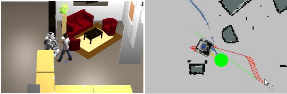
Fig. 9. Narrow passage passing scenario. In this scenario, human and robot arrive at the common passage at the same time, and one should back off to provide way to another. Otherwise, there exists no solution. This is one of the intricate situations addressed in this work, and the picture on the left shows the simulation of this scenario in MORSE [22]. Right side picture shows the trajectories for the human (blue) and the robot (red), generated using the proposed framework, HATEB-2. It can be seen from the picture that the robot’s trajectory (red) is making the robot to move backwards and hence providing way to the human.
