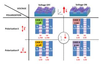
**Fig. 3.** Scheme of the different situations according to the incident polarization and the applied voltage governing the LC orientation.
