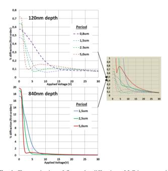
**Fig. 6.** Characterization of first order diffraction of LC-impregnated cells illuminated with a S-polarized incident beam depending of the applied electric field for various grating periods (purple to red lines) at depths of 120 (dashed lines on the top) or 840nm (plain curves below). Inset: comparison for all periods and depths to show the maximal extinction of diffraction occurs at the same level ( $\approx 0.1\%$ ).
