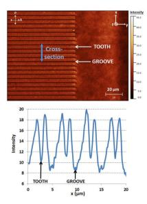
**Fig. 8.** Microscopic observation (x50) between cross polarizers of LC-impregnated diffraction gratings (5.0 $\mu$ m period and 840nm depth) with a tension of 10V applied in the cell (at the top). A cross section show the repartition of the birefringence in teeth/groove interfaces (below).
