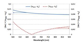
**Fig.11.** Difference between the ULIS resin refractive index and liquid crystal E7 considering extraordinary index (blue plain line, left Y axis) and ordinary index (red dashed line, right Y axis). Refractive index of ULIS resin was measured by ellipsometry while E7 liquid crystal dispersion curves are derived from extended experimental measurements by a three-coefficient Cauchy model (Li and al. 2005).
