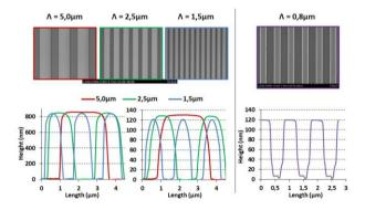
**Fig. 2.** SEM images (upper part) and AFM characterizations (lower part) of gratings from 0.8 to 5.0μm fabricated by photolithography (left) or by nano-imprint lithography (right).
