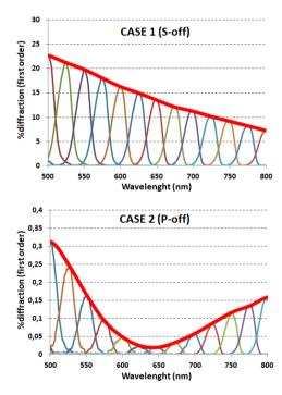
**Fig.10.** First order's diffraction spectrum (in red, bold) obtained as the envelope of the experimental measurements at different diffraction angles (fine colors). LC-impregnated grating with 1.5µm period and 840nm deep is illuminated with a S-polarized incident beam (at the top) and P-polarized light (bottom) without applied voltage.
