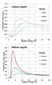
**Fig. 7**. Characterization of first order diffraction of LC-impregnated cells illuminated with a P-polarized incident beam depending of the applied electric field for various grating periods (purple to red lines) at depths of 120 (dashed lines on the top) or 840nm (plain curves below).
