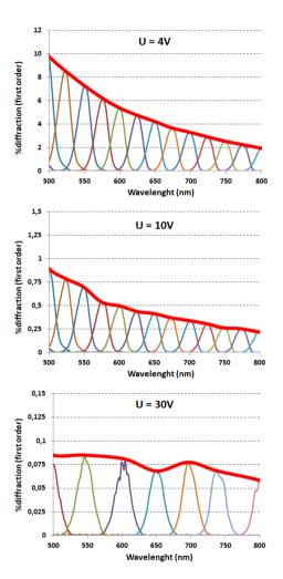
**Fig.12**. First order diffraction spectrum (in red, bold) obtained as the envelope of the experimental measurements at different diffraction angles (fine colors). LC-impregnated grating with 1.5μm period and 840nm deep is illuminated with a S-polarized incident beam and various applied voltages: 4V (above), 10V (middle), 30V (bottom).
