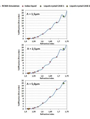
**Fig. 4.** First-order diffraction measurements on cells with 840nm depth gratings impregnated with various index liquids (red circles), liquid crystals in S or P-polarizations (green or yellow diamonds) compared to RCWA simulations (blue curve).
