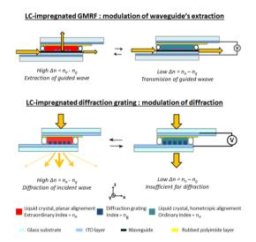
**Fig. 1.** Schematic view of the principle of modulation of waveguide's extraction by LC-impregnated GMRF (above) and modulation of diffraction by LC-impregnated grating (below). In both cases, the diffractive state  $(\Delta n = n_e - n_g)$  is represented in left and the non-diffractive state  $(\Delta n = n_o - n_g)$  in right.
