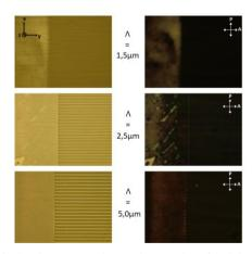
**Fig. 5.** Optical microscopy observation (x50) of LC-impregnated diffraction gratings with period from 1.5 to 5.0μm and 840nm depth without polarizers (in left) and between cross polarizers (in right). As expected for aligned LCs, transmission is extinguished between crossed polarizers.
