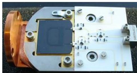
Figure 12: Full cryogenic HTS oscillator with output buffer (B type). Superconductor resonator on the left and active circuit on the right side.
