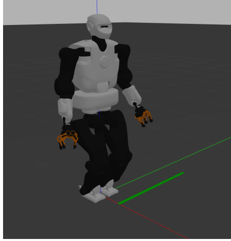
Figure 17: Initial state of Pyrène in simulation with a stick as obstacle, 25cm ahead of him, 4mm high and 3cm large. In this configuration, Pyrène steps on it with the tip of the left foot at its second foot step.
