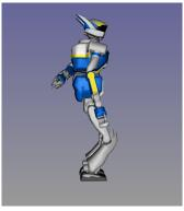
Fig. 9. Constrained motion planning for HRP-2 humanoid robot sliding on the ground in quasi-static equilibrium: the feet should stay horizontal with a fixed relative position and the center of mass should project between the feet. The initial configuration is shown on the left. The goal configuration is shown on the right. The algorithm is a constrained RRT close to the one described in Dalibard *et al* [16]
