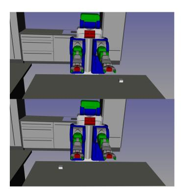
Fig. 11. Manipulation planning problem with PR-2 robot manipulating a box. The robot needs to flip the box upside down from an initial pose (top) to a goal pose (bottom).
