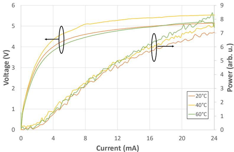
Figure 6. L-I-V characteristics of 50μm-wide-apertured VCSELs as a function of temperature
