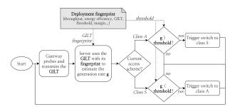
Fig. 1: TREMA's switching mechanism flowchart
