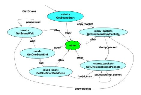
Figure 11: Finite-state machine of the GetScans activity (Listing 8)
