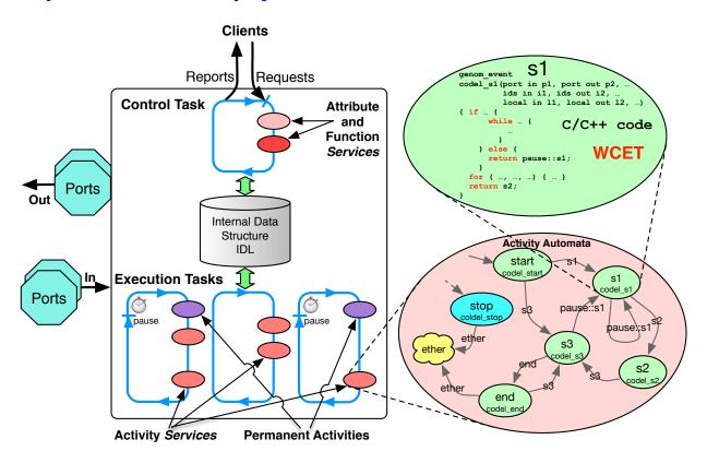
Figure 10: A G<sup>en</sup> M generic functional component (module).
