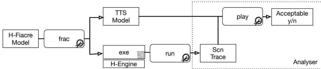
Figure 6: Scheme of the acceptance test for traces.
