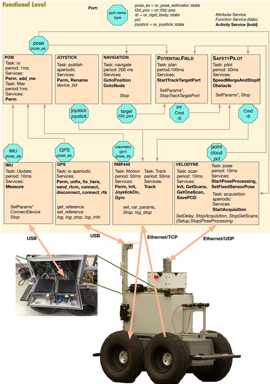
Figure 9: Architecture of the Minnie RMP440 experiment.
