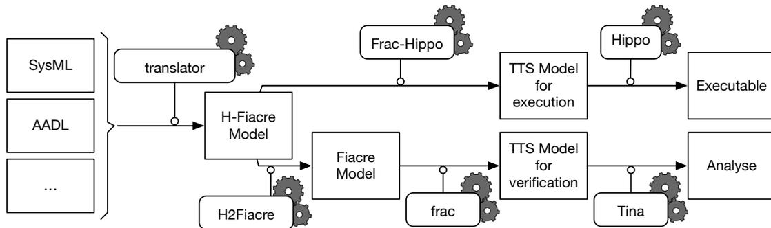
Figure 2: A schematic representation of the HIPPO toolchain.
