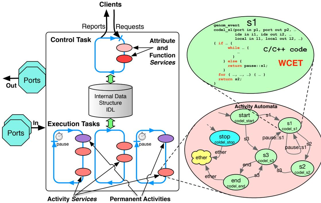
Figure 10: A  $G^{\text{en}}\%M$  generic functional component (module).
