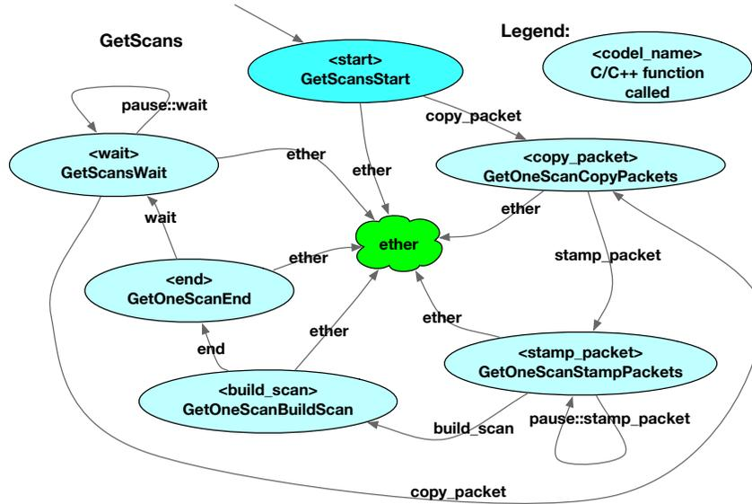
Figure 11: Finite-state machine of the *GetScans* activity (Listing 8). Each state is labeled with its name between `<>` and its codel (the C/C++ function called). Transitions are labeled with the name of the next state (i.e. the returned value from the originating state codel).
