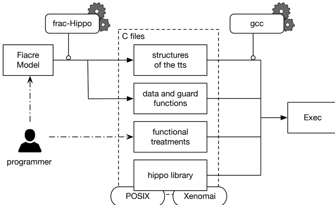
Figure 4: Tools for code generation and compilation.
