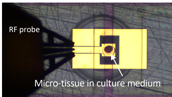
Fig. 6. Photography of an RF applicator under test, loaded with a micro-tissue.
