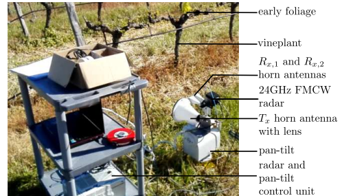
Fig. 1. Ground-based FM-CW radar performing a beamsweeping in front of a vineplant. The photograph has been taken in May 2017 and, as observed, the foliage of the vineplants starts to grow.
