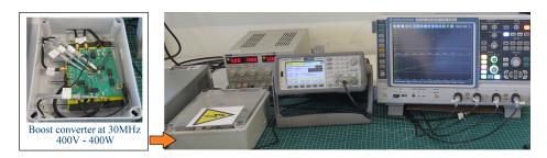
Figure 20: Experimental setup boost converter 400V - 400W at 30MHz.
