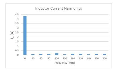
Figure 4: Current harmonic spectrum for the studied inductor.
