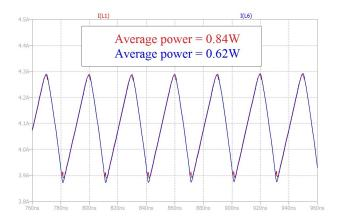
Figure 12: Inductor current. Color nomenclature: blue – ideal inductor with low series resistance, red – power inductor considering  $Q(30\mathrm{MHz})=100$  and  $SRF=250\mathrm{MHz}$ .
