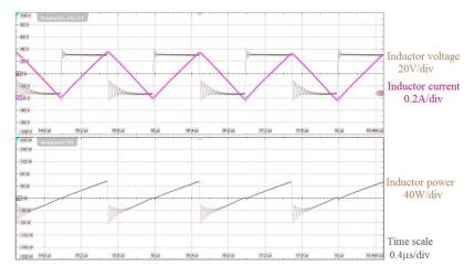
Figure 17: Experimental results for 1MHz boost converter. Inductor SRR1210-8R2.  $P_{avg}$ =492mW.
