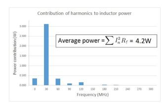
Figure 7: Inductor power in the frequency-domain.
