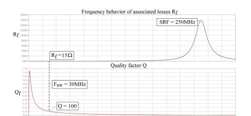
Figure 11: Frequency behavior of  $R_f$  and  $Q_f$  for the modeled inductor.
