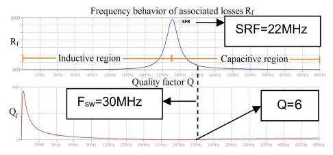
Figure 2: Frequency behavior of  $R_f$  and  $Q_f$  for the power inductor used in the designed boost converter.
