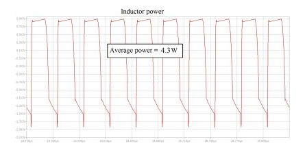
Figure 6: Inductor power in the time-domain.
