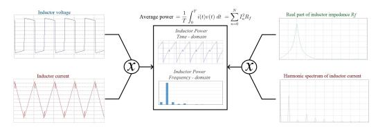
Figure 5: Extension of Parseval's theorem for the inductor analysis in power converters.
