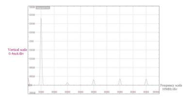
Figure 16: FFT of inductor current for test at  $10 \mathrm{MHz}$  - square signal. Inductor reference SRP5015A.
