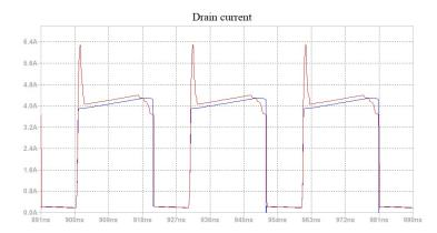
Figure 10: Impact of the SRF on the drain current. Color nomenclature: blue - drain current for SRF=250MHz, red - drain current for SRF=30MHz.
