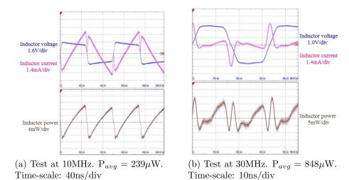
Figure 15: Test inductor SRP5015A at 10MHz and 30MHz.
