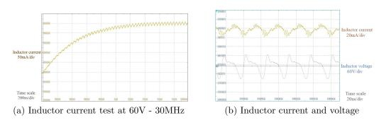
Figure 19: Inductor current and voltage for boost converter 60V - 10W at 30MHz
