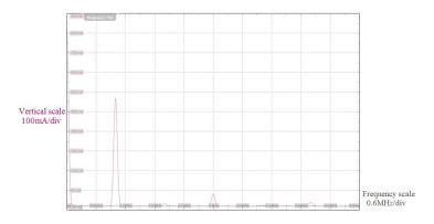
Figure 18: FFT for the inductor current of 1MHz boost converter.
