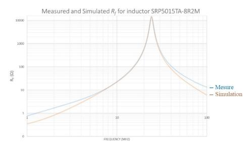
Figure 14: Real part of inductor impedance  $(R_f)$ . Inductor reference SRP5015TA-8R2M.
