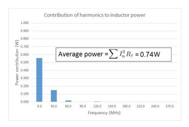
Figure 13: Inductor power distribution in the frequency-domain for Q(30 MHz)=100 and SRF=250 MHz.
