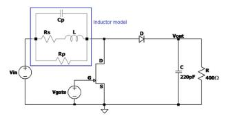
Figure 9: Boost converter with inductor model.
