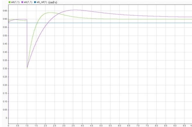
Figure 3: Real time trajectories of the rotation speeds  $\omega_b$  for the non linear system (1) with previous hypothesis (theoretical trajectory in blue, manually tuned controller in purple, multi objective controller in green).
