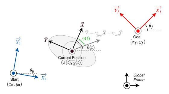
Figure 2. Coordinate systems in the trajectory problem to solve
