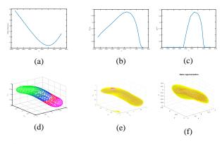
Fig. 3: (a) Miss distance (m) (b) Instantaneous collision probability  $\mathcal{P}(t)$  with (c) and without (d) velocity uncertainty (d) 3D Swept-volume shape (no velocity uncertainty) (e) PSS approximation d=8 (f) Projection of 6D PSS approx, d=8, for a fixed mean velocity.
