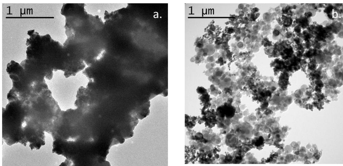
**Figure 24:** TEM images of nanocomposites made by direct mixing of Al and CuO nanoparticles (a), and assembled with optimized and complementary DNA strands (b).
