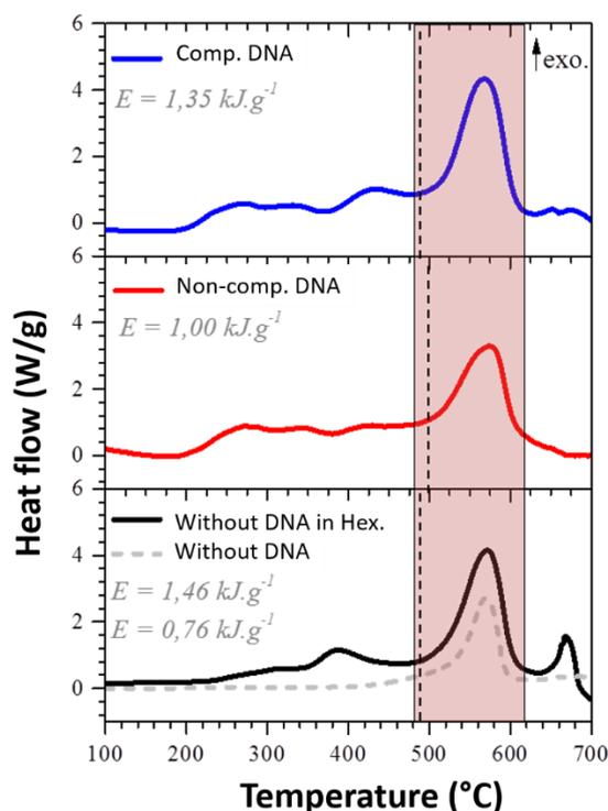
**Figure 23:** DSC curves of different Al-CuO nanobiocomposites obtained by assembly of Al and CuO nanoparticles with optimized and complementary DNA strands (blue curve), optimized and non-complementary DNA strands (red curve) and non-complementary functionalized DNA strands in aqueous solution (black curve) or in hexane (dashed grey curve).
