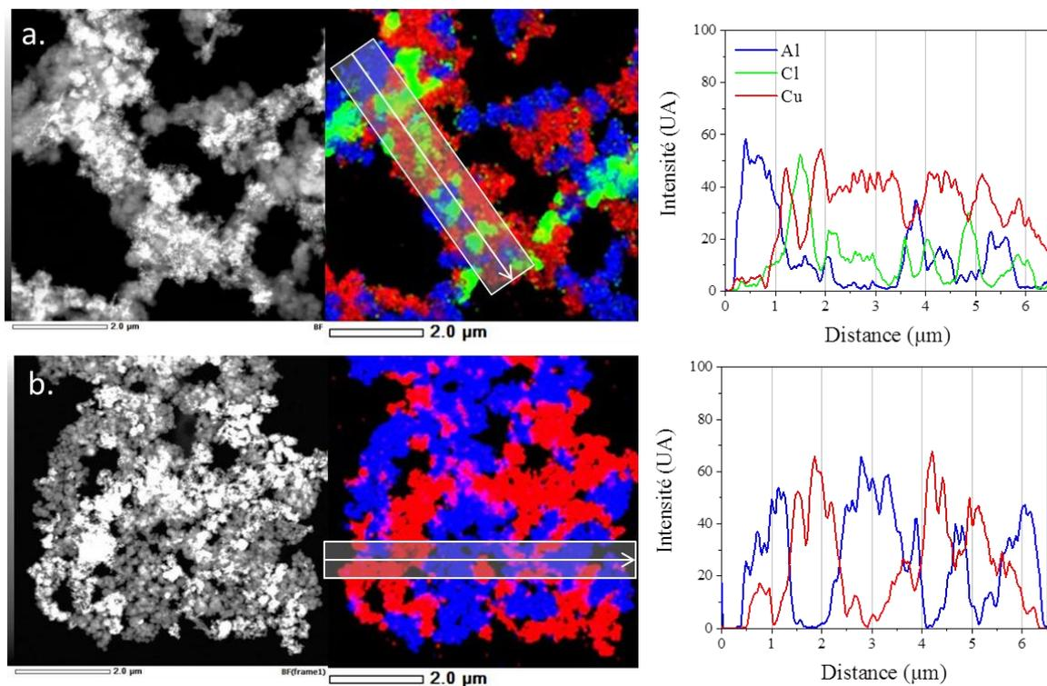
**Figure 25:** Dark film TEM images; elemental maps of Al (blue), Cu (red) and Cl (green); and elemental composition of a slice of Al-CuO nanocomposites obtained by aggregation of Al and CuO nanoparticles without DNA (a) and by assembly with optimized and complementary DNA strands (b).
