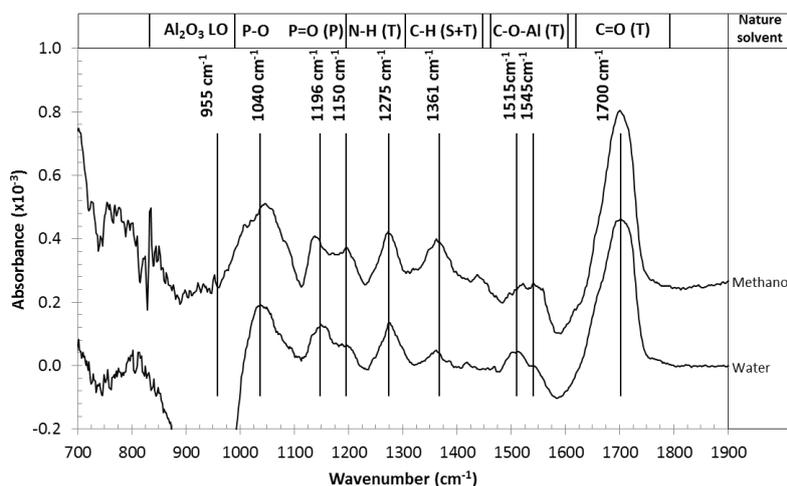
**Figure 18:** Influence of the nature of the solvent on the IR absorbance spectra of an alumina surface after dTMP deposition. The incubation of the surface was performed using methanol (top curve) and water (bottom curve) with the same concentration of dTMP to a clean alumina substrate in both cases. Related dTMP regions are reported on the top of the figure: T for thymine, S for sugar, and P for phosphate according to assignments resulting from DFT calculations.<sup>100</sup>
