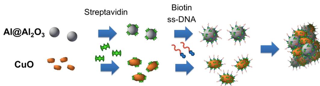
**Figure 13.** Illustration of the functionalization process developed to enable the DNA-directed self-assembly of core-shell Al (Al covered with Al<sub>2</sub>O<sub>3</sub> shell) and CuO nanoparticles.
