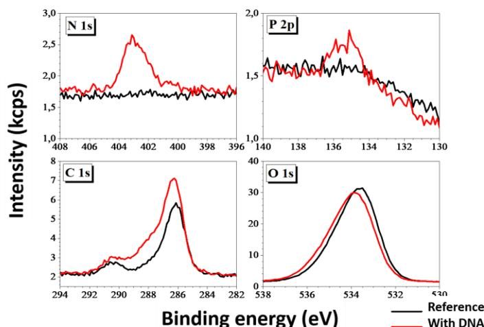
**Figure 17:** XPS spectra for three primary elements in *dTMP* deposited on alumina surface. The black curve corresponds to the signal of the reference (alumina substrate), while the red curve corresponds to the alumina surface with deposited *dTMP*.<sup>100</sup>
