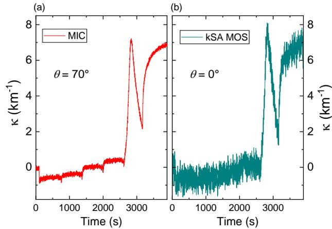
**Figure 6.** Curvature changes during a sequence of growths and growth stops of sputter-deposited Ag on a-Si as a function of time measured simultaneously with our MIC-based setup (a) and a commercial laser deflectometry-based tool (b). The MIC-based setup was mounted on the  $70^\circ$  viewports of the magnetron sputtering chamber while the kSA MOS was mounted at normal incidence ( $\theta = 0^\circ$ ).
