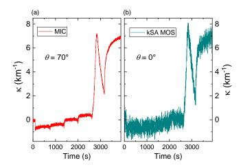
**Figure 6.** Curvature changes during a sequence of growths and growth stops of sputter-deposited Ag on a-Si as a function of time measured simultaneously with our MIC-based setup (a) and a commercial laser deflectometry-based tool (b). The MIC-based setup was mounted on the 70° viewports of the magnetron sputtering chamber while the kSA MOS was mounted at normal incidence ( $\theta = 0^{\circ}$ ).
