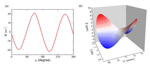
**Figure 3.** The curvature measured on a bare 50 mm diameter, 350  $\mu$ m thick GaAs (001) oriented wafer while rotating at 12 rpm around its axis, at 580°C (a) allows for its complete shape reconstruction in real-time (b).
