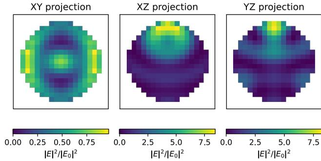
Figure D.20: Graphical output of the example script given in listing 1. A dielectric sphere ( $n = 2$ ,  $r = 160$  nm) in vacuum is illuminated from below by a plane wave of linear polarization along  $X$  and wavelength  $\lambda_0 = 400$  nm. Each plot shows the E-field intensity inside the sphere on a slice through its center on an area of  $400 \times 400$  nm<sup>2</sup>.
