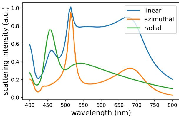
Figure 16: Scattering from a silicon nanosphere of diameter  $D = 170$  nm in oil ( $n_{\text{oil}} = 1.48$ ), illuminated by different polarized vectorbeams through a numerical aperture of  $NA = 1.2$ . The blue line corresponds to a linear polarized  $TEM_{00}$  beam, the orange line to azimuthal polarization and the green line to radial polarization.
