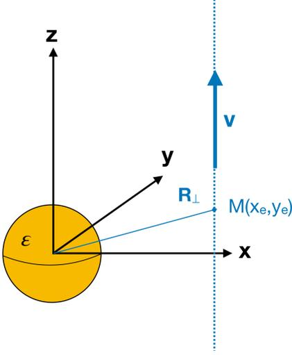
Figure C.19: A fast electron is incident on a nanostructure and crosses the (OXY) plane at  $\mathbf{R}_\perp = (x_e, y_e)$ . We compute the electron energy losses experienced by the swift particle in the framework of the Green Dyadic Method.
