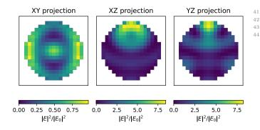
Figure D.20: Graphical output of the example script given in listing 1. A dielectric sphere (n = 2, r = 160 nm) in vacuum is illuminated from below by a plane wave of linear polarization along X and wavelength  $\lambda_0 = 400 \text{ nm}$ . Each plot shows the E-field intensity inside the sphere on a slice through its center on an area of  $400 \times 400 \text{ nm}^2$ .
