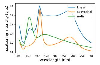
Figure 16: Scattering from a silicon nanosphere of diameter  $D = 170 \,\mathrm{nm}$  in oil  $(n_{\mathrm{oil}} = 1.48)$ , illuminated by different polarized vectorbeams through a numerical aperture of NA = 1.2. The blue line corresponds to a linear polarized TEM<sub>00</sub> beam, the orange line to azimuthal polarization and the green line to radial polarization.
