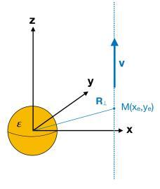
Figure C.19: A fast electron is incident on a nanostructure and crosses the (OXY) plane at  $\mathbf{R}_{\perp} = (x_e, y_e)$ . We compute the electron energy losses experienced by the swift particle in the framework of the Green Dyadic Method.
