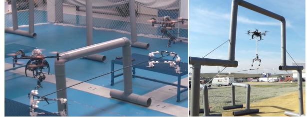
Fig. 7: Two aerial manipulators assembling a structure (left). Long reach aerial manipulator with dual arm transporting a bar (right).
