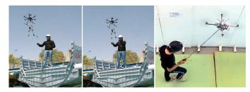
Fig. 8: AEROM providing a tool (left) and guiding a human (right).
