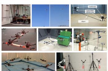
Fig. 4: Examples of aerial cooperative manipulation systems (from top, from left): 1) multi-quadrotor cable-suspended transport [7]; 2) multi-helicopter cable-suspended transport [12]; 3) cooperative aerial manipulators [128]; 4) rigidly-attached quadrotors [129]; 5) SmQ platform [130]; 6) MAGMaS platform [101]; 7) flexible ring cooperative manipulation [131]; and 8) distributed vibration suppression with RVMs [132].
