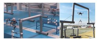
Fig. 7: Two aerial manipulators assembling a structure (left). Long reach aerial manipulator with dual arm transporting a bar (right).
