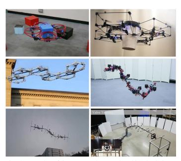
Fig. 5: Examples of interconnected actuated multi-body designs (from top, from left): 1) HYDRUS [105]; 2) flying-gripper [146]; 3) distributed flight array (DFA) [147]; 4) DRAGON [148]; 5) flying LASDRA [149]; and 6) operation LASDRA [109].
