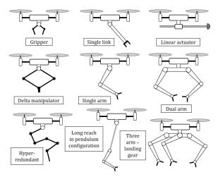
Fig. 3: Different morphologies of aerial manipulation robots.
