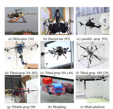
Fig. 2: A representative example for each type of multi-rotor platforms employed for physical interaction.
