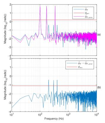
Fig. 10: Simulated result of SC-TFSP in case of target motion composed of tones of 4 µm amplitude at 100 Hz, 170 Hz and 340 Hz, and tones of 25 nm amplitude at 200 Hz, 300 Hz and 400 Hz. (a) Spectrum (blue) of  $\hat{\phi}_F$  and  $\hat{\phi}_{F\_new}$  (magenta) alongside primary threshold (red). (b) Spectrum (blue) after the subtraction alongside secondary threshold (red).
