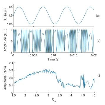
Fig. 9: Simulated result of SC-TFSP in case C varies by 10% in a sinusoidal manner at the main-tone frequency of 170 Hz with mean C value of 1.5 while target motion is composed of a main tone  $\phi_{main}$  at 170 Hz with amplitude of 2 µm and another tone of 10 nm amplitude at 20 Hz with  $\alpha = 5$ , and  $F_s = 1$  MSPS: (a) Time-variation in C, (b) original SM signal  $P_{org}(t)$ , and (c) amplitude of secondary harmonic vs  $\hat{C}_a$ .
