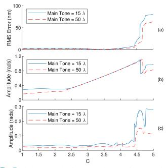
Fig. 7: Simulated result of SC-TFSP in case of target motion composed of main tone  $\phi_{main}$  of  $15\lambda$  (blue line) and  $50\lambda$ (dashed line in red) amplitudes at 170 Hz and another tone of 10 nm amplitude at 20 Hz with  $\alpha = 5$  sampled at 10 MSPS. (a) RMS error in main tone vs C. (b) Amplitude of secondary harmonic in the spectrum of  $\hat{\phi}_F$  vs C. (c) Amplitude of secondary harmonic in the subtracted spectrum with  $\hat{C}$  assigned the value equal to C vs C.
