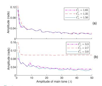
Fig. 6: Effect of increase in  $F_s$  from 1 MSPS to 10 MSPS on amplitude of secondary harmonic in the subtracted spectrum with  $\hat{C}$  assigned the value  $\hat{C}_a$ . All other parameters remain the same as reported in caption of Fig. 5.
