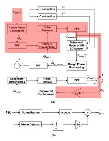
Fig. 2: Schematic diagram of (a) proposed spectral subtraction based TFSP (SC-TFSP), where original TFSP [25] is shaded in red, and (b) rough phase unwrapping.
