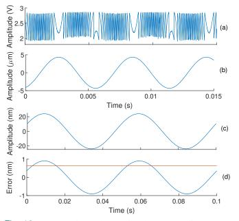
Fig. 12: (a) Experimental SM signal corresponding to PZT target vibration consisting of a main tone with 4.4  $\mu$ m amplitude at 170 Hz and a small tone with 25 nm amplitude at 20 Hz, (b) recovered main tone, (c) recovered small tone, and (d) error between PZT based small tone and recovered small tone (blue), and its RMS value (red).
