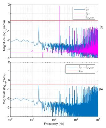
Fig. 11: Experimental result of proposed SC-TFSP in case of PZT target motion composed of a tone of 4.4  $\mu$ m amplitude at 170 Hz and another tone of 25 nm amplitude at 20 Hz. (a) Spectrum (blue) of feedback phase  $\hat{\phi}_F$  recovered from experimental SM and Spectrum (magenta) of feedback phase  $\hat{\phi}_{F\_new}$  of generated SM signal signal alongside primary threshold (red). (b) Spectrum (blue) after the subtraction alongside secondary threshold (red).
