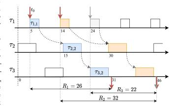
Fig. 1. Task chain run-time example with  $\tau_1 \to \tau_2 \to \tau_3$
