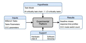
Fig. 5. Experimental Platform structure
