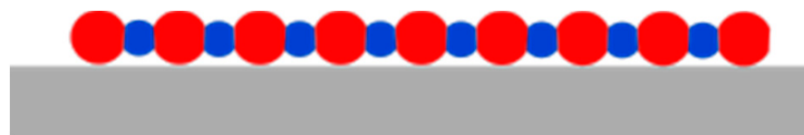
Figure 2. Schematic of an alternating chain of reactant particles from which an effective conduction coefficient is derived.
