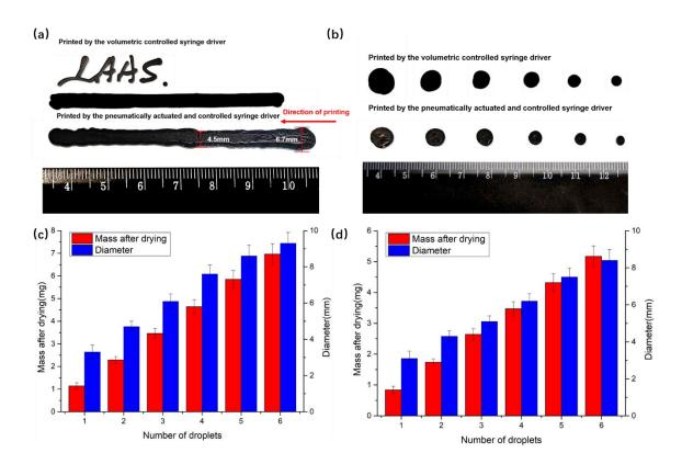
**Figure 6.** (a) Representative photographs of linear writing and (b) dropwise writing results obtained using the volumetrically controlled dispenser and pneumatically actuated syringe. Average diameter and mass of the droplets printed (c) with volumetrically controlled dispenser and (d) with pneumatically actuated syringe as a function of droplets.
