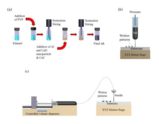
**Figure 1.** Schematic of (a) the thermite composites and inks preparation and direct-writing methods with (b) a simplest pneumatically actuated syringe, and with (c) the volumetrically controlled dispenser.
