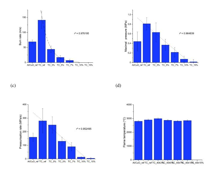
**Figure 4.** (a) Burn rate, (b) maximal pressure, (c) pressurization rate and (d) flame temperature as a function of the PVP content.
