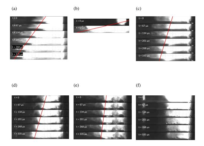
**Figure 5.** High-speed video images recorded for (a) Al/CuO\_ref, (b) TC\_ref, (c) TC\_3%, (d) TC\_5%, (e) TC\_7%, (f) TC\_10%. Each image is composed of 6 frames separated by 67 μs except for TC\_ref which burns faster and contains only 2 frames. Total burning length is 3 cm.
