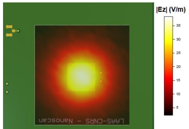
Fig. 5. Electrical near-field map at 10 mm above island P1 (excitation frequency = 10 MHz)
