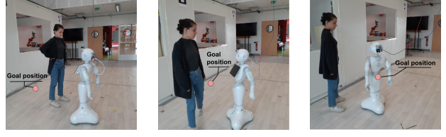
(a) Human who put themselves on the robot path, preventing the robot to navigate towards its goal position (b) Human who put themselves on the robot path after it computed a new path to reach its goal position (c) Human finally getting outside of the robot path, allowing it to reach its goal position
