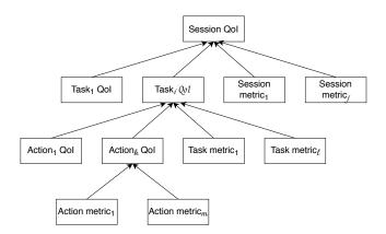
Fig. 2: Representation of the QoI dependencies, with i the number of performed tasks during the interaction session, k the number of performed actions during the task i, j the number of metrics to measure the interaction session QoI, l the number of metrics to measure the task i QoI and m the number of metrics to measure the action k QoI.
