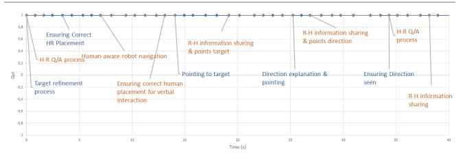
(a) Evolution over time of the measured QoI for the 'ideal' human. Both action and task QoIs remain at 1 as the task is proceeding smoothly.
