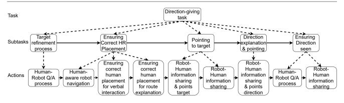
Fig. 8: The representation of the direction-giving task as a hierarchical task network with task, substasks and actions levels. All the horizontal arrows are sequential links and the rest are decomposition ones.
