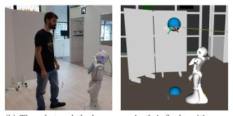
(b) The robot and the human are in their final positions as planned by the robot. The blue spheres are the computed position for the human by the robot. The robot is pointing at the place direction.
