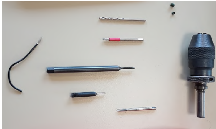
FIGURE 2.9 – Outils de pose des helicoils
