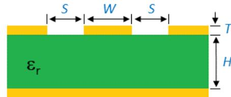
**Fig. 8:** Parameters of coplanar transmission line.
