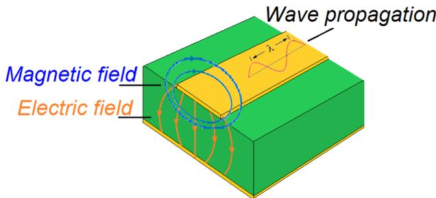
Fig. 1: Transmission line model of a PCB trace.
