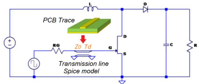
Fig. 3: High-frequency boost converter with transmission line model.
