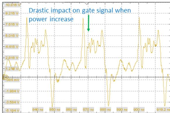
**Fig. 15:** Gate signal at high output power.
