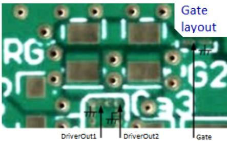
Fig. 11: PCB layout around the gate driver.
