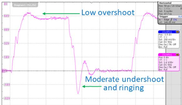
**Fig. 14:** Gate signal at low output power.
