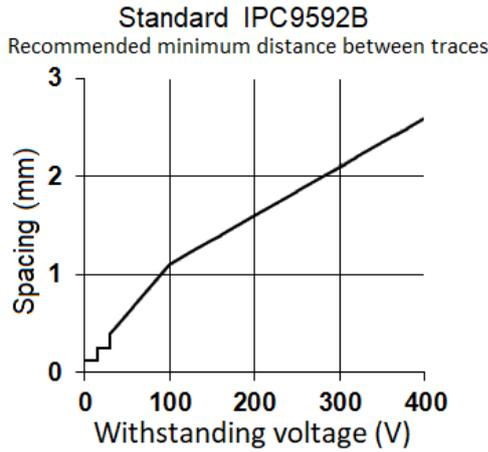
Fig. 10: Minimum trace spacing according to IPC9592B
