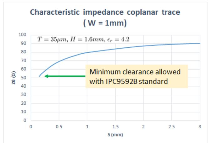
**Fig. 9:** Characteristic impedance of coplanar transmission line.
