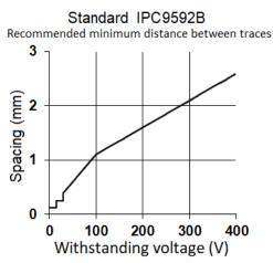
Fig. 10: Minimum trace spacing according to IPC9592B
