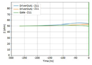
Fig. 13: Characteristic impedance measurement of PCB gate layout. Negative time corresponds to reflected measure signals.
