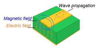
Fig. 1: Transmission line model of a PCB trace.
