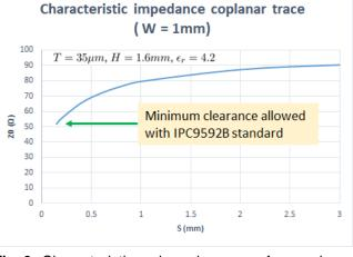
Fig. 9: Characteristic impedance of coplanar transmission line.
