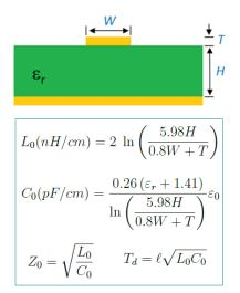
**Fig. 2:** Characteristic impedance  $Z_0$  and propagation time  $T_d$  from PCB parameters.
