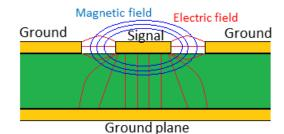
Fig. 7: Magnetic and electric fields in coplanar transmission line.
