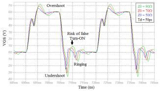
Fig. 4: Simulations results of boost converter with transmission line model in the gate path.
