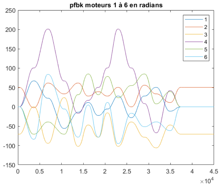
Figure 3.11: Motor angles measured at 5 kHz
