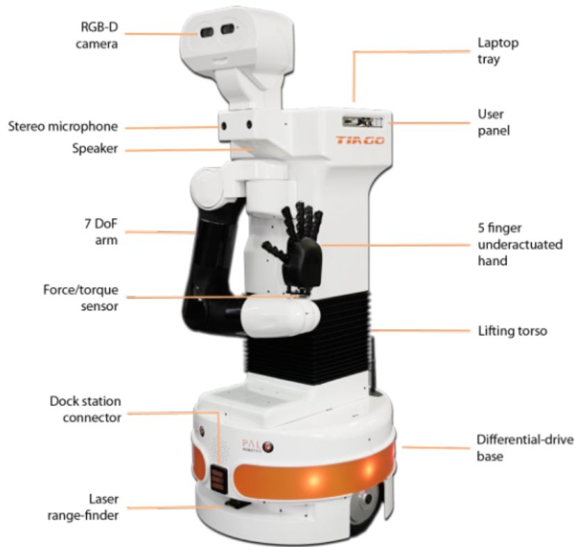
Figure 3.17: TIAGo robot main components
