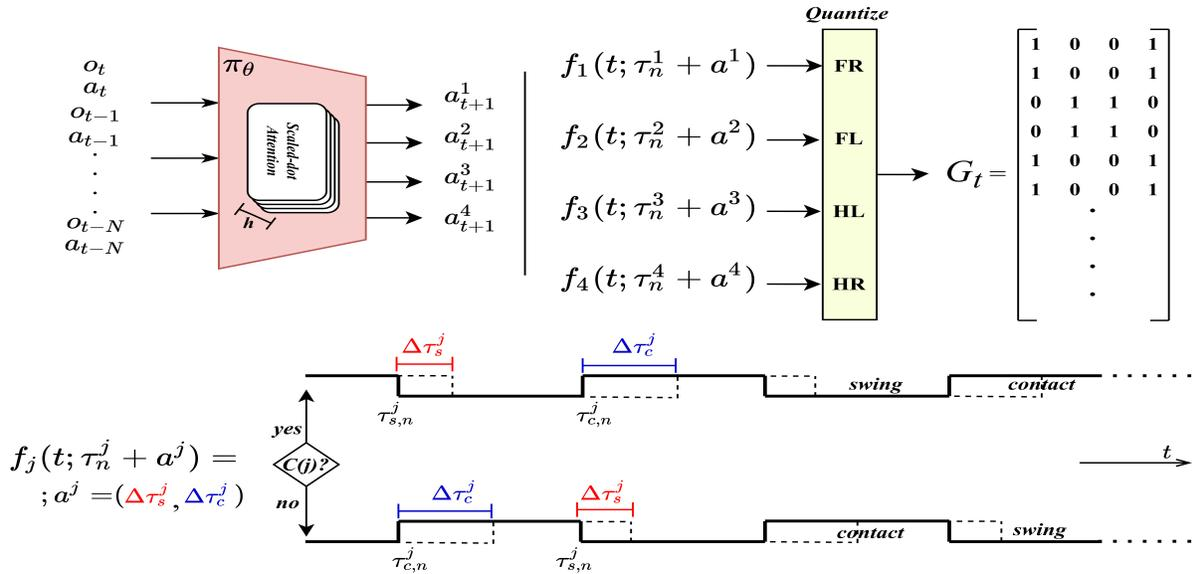
Fig. 2: Multi-headed self-attention layers, with  $h = 8$  heads, are used as the base of the policy. The actions modify the contact sequence given by the oscillations of each leg. The bottom plot shows an example of the nominal sequence of contact/swing in bold. Depending on the current contact state of foot  $j$ , the dotted line draws the new oscillation after the shifts in timings given by the policy are taken into account.
