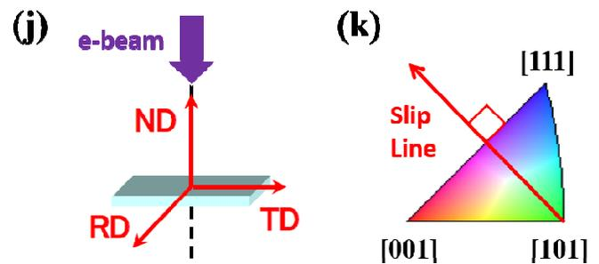
Fig. 3. EDM images taken for the non-annealed (i.e., (a), (b), and (c)) and the annealed Cu thin films. UV NLA was at  $LF_1$  for  $t_2$  ((d), (e), and (f)) or  $t_4$  ((g), (h), and (i)). As depicted in (j), ND, TD, and RD stand for Normal Direction, Transverse Direction, and Reference Direction, respectively. Also, a standard triangle of grain orientations is also shown in (k).
