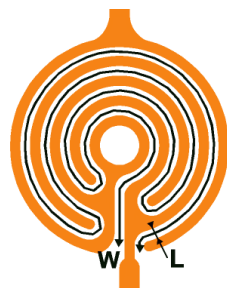
Figure 2. Structure of the comb-shaped sensing electrodes.
