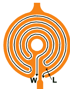
Figure 2. Structure of the comb-shaped sensing electrodes.
