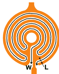
Figure 2. Structure of the comb-shaped sensing electrodes.
