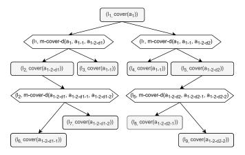
Fig. 2. Grounded HTN tree for the problem listed in Listing 2. Rounded rectangles represent labeled tasks (in  $V_T$ ), hexagons represent labeled methods (in  $V_M$ ).
