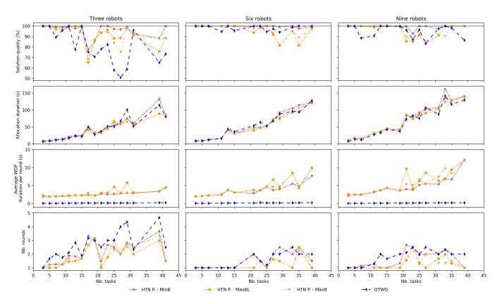
Fig. 3. Results for unordered HTNs showing the quality (top), allocation duration (2nd row), WDP duration (3rd row) and number of necessary rounds (bottom) for 3, 6 and 9 robots (respectively left, middle, and right columns). The three *MinB*, *MaxB*, and *MaxBL* approaches are compared to the centralized reference (continuous line) and the *OTWD* algorithm.
