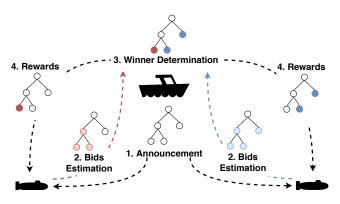
Fig. 1. Overview of the approach. The whole mission decomposed as a HTN is auctioned. Each robot bids on the sub-tasks, a winner determination process allocates the tasks and sends them to the robots ("rewards").
