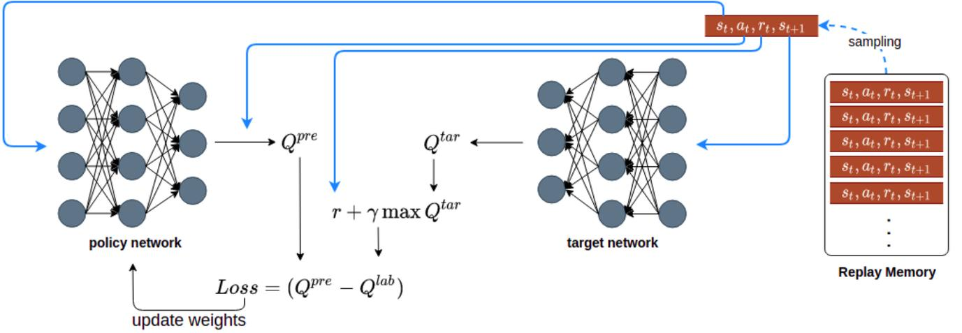
Fig. 2. Double Deep Q-Network-based agent structure
