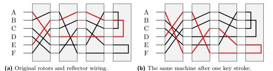
**Figure 1** Illustration of Enigma's rotors and reflector.
