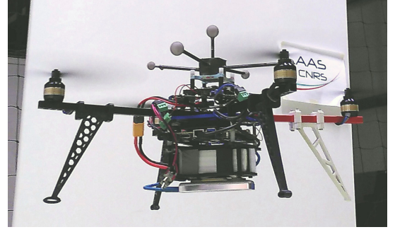
Fig. 3: One of the quadrotors used in the presented experiment.
