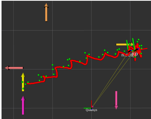
Fig. 8. Visualization of the recorded data on Rviz (in red the MoCap set and in green the ICP set)
