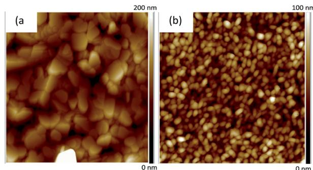
Fig. 3 AFM tapping mode (a)  $5 \times 5 \mu\text{m}^2$  image of 75 nm tetracene and (b)  $2 \times 2 \mu\text{m}^2$  image of 50 nm benzo-hexacene films grown on SiO<sub>2</sub>/OTS substrates at a deposition flux of *ca.*  $0.4 \text{ \AA s}^{-1}$ .
