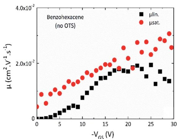
Fig. 7 Mobility vs.  $V_{GS}$  in linear (black,  $V_{DS} = -10$  V) and saturation (red,  $V_{DS} = -50$  V) regimes for the no-OTS benzo[hexacene] based transistor with channel size  $W/L = 1000 \mu\text{m}/50 \mu\text{m}$ .
