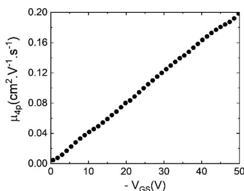
Fig. 8 Four-probe mobility vs.  $V_{GS}$  (calculated according to eqn (1)) in the linear regime ( $V_{DS} = -10$  V) for the no-OTS benzo[hexacene] based transistor with channel size  $W/L = 300 \mu\text{m}/200 \mu\text{m}$ .
