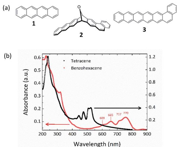
Fig. 2 (a) Chemical structure of the materials used in this study: 1, tetracene; 2 benzo-hexacene precursor; 3, benzo-hexacene after decarbonylation of 2. (b) Absorption spectra of tetracene and benzo-hexacene evaporated thin films.
