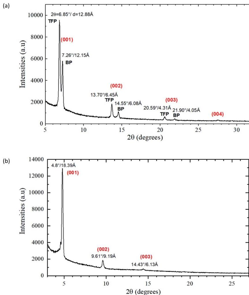
Fig. 4 X-ray diffraction patterns of the (a) SiO<sub>2</sub>/OTS/tetracene (75 nm) and (b) SiO<sub>2</sub>/OTS/benzohexacene (50 nm) samples.
