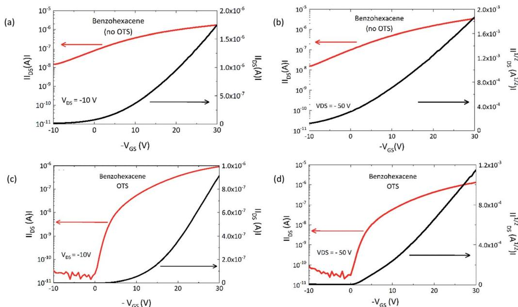
Fig. 6 Semilogarithmic transfer curves (left y-axis) and plot of square root ( $I_{\text{DS}}$ ) (right y-axis) versus gate voltage for (a and c)  $V_{\text{DS}} = -10 \text{ V}$  and (b and d)  $V_{\text{DS}} = -50 \text{ V}$  of the no OTS and OTS-grafted benzohexacene based transistor with channel size  $W/L = 1000 \mu\text{m}/50 \mu\text{m}$ .
