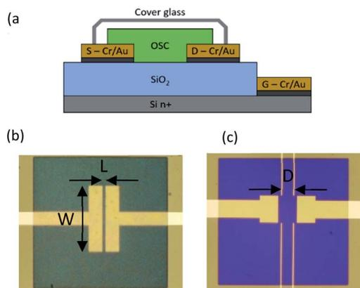
Fig. 1 (a) Schematic representation of the bottom gate bottom contact OTFT and pictures of OTFTs with (b) tetracene 2-probe  $W = 1000 \text{ }\mu\text{m}$  and  $L = 50 \text{ }\mu\text{m}$  and (c) benzohexacene 4-probe devices  $D = 80 \text{ }\mu\text{m}$ .
