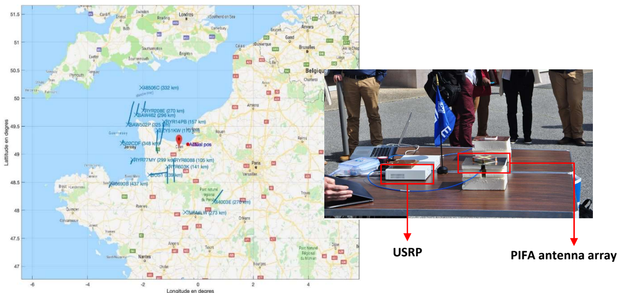
Figure 11: Real time trajectory on the map of the detected aircrafts and a photo of the antenna during tests at the contest.
