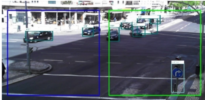
Fig. 4. Object detection in urban settings. Each bounding box has a label that identifies the type of object and the confidence score of the detection. The annotated images are streamed by a webserver.
