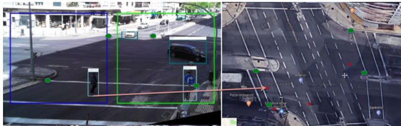
Fig. 6. Green dots are used to compute the transformation between cameras. Red dots represent the predicted location of the midpoint of the bounding box low segment
